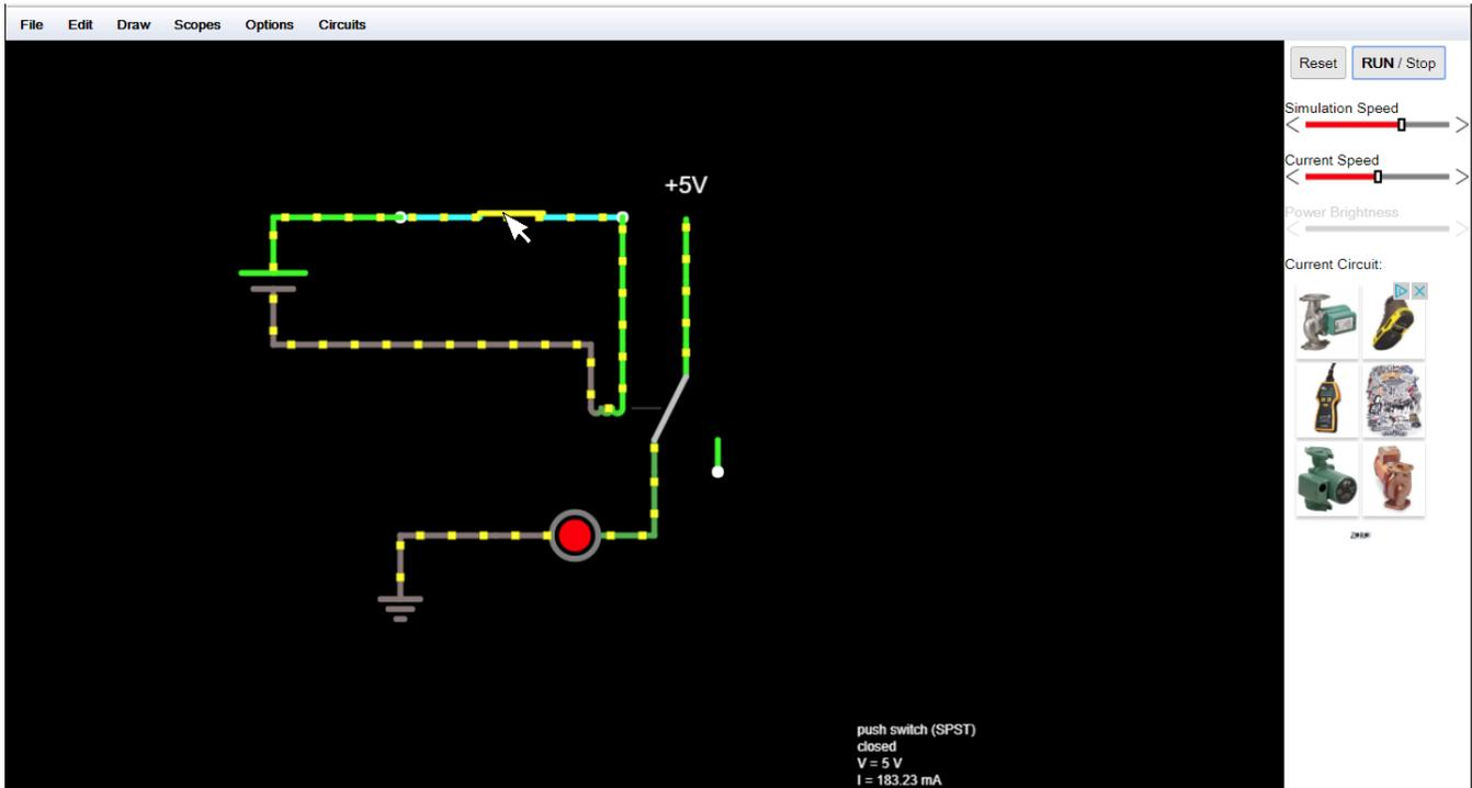
Changing the state of the switch will cause the LED to turn on and off (the circle will be black or red unless you have changed the LED properties). In addition to the LED lighting up, you will see a current being simulated via the yellow dots moving around the complete(d) circuit(s).
