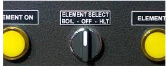
Figure 12. An example of a 3 position (multiple throw) selector switch.
