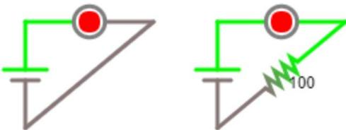
Figure 15. Circuit without (left) a resistor and one with (right) a resistor.
