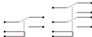
Figure 3. SPDT relay (left) and DPDT relay (right)
